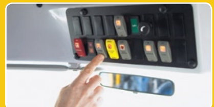
Driver switches located overhead for easy access and enhanced loading visibility.
